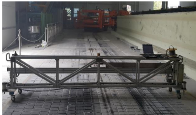
Figure 4. Transverse profile logger.
