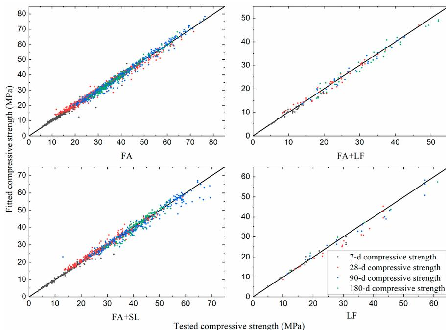
**Figure 3.** Relationship between tested compressive strength and fitted concrete compressive strength.
