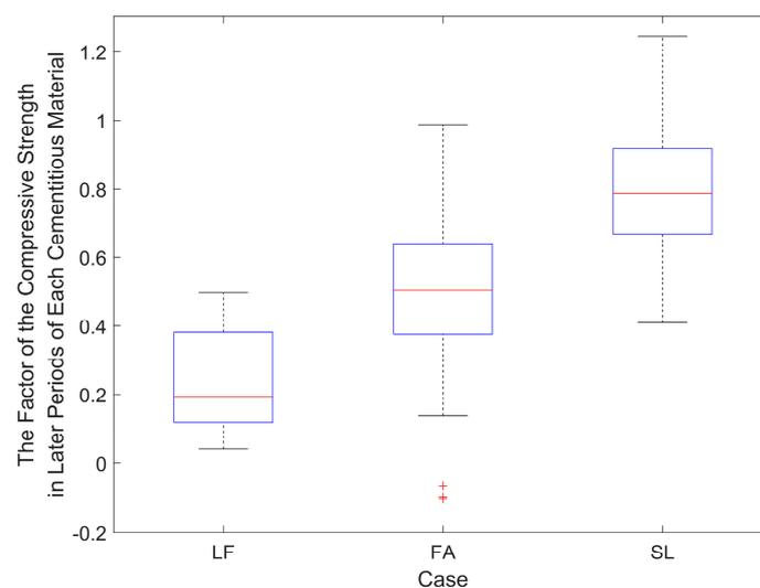
Figure 6. The factor of the compressive strength in later periods of each cementitious material.
