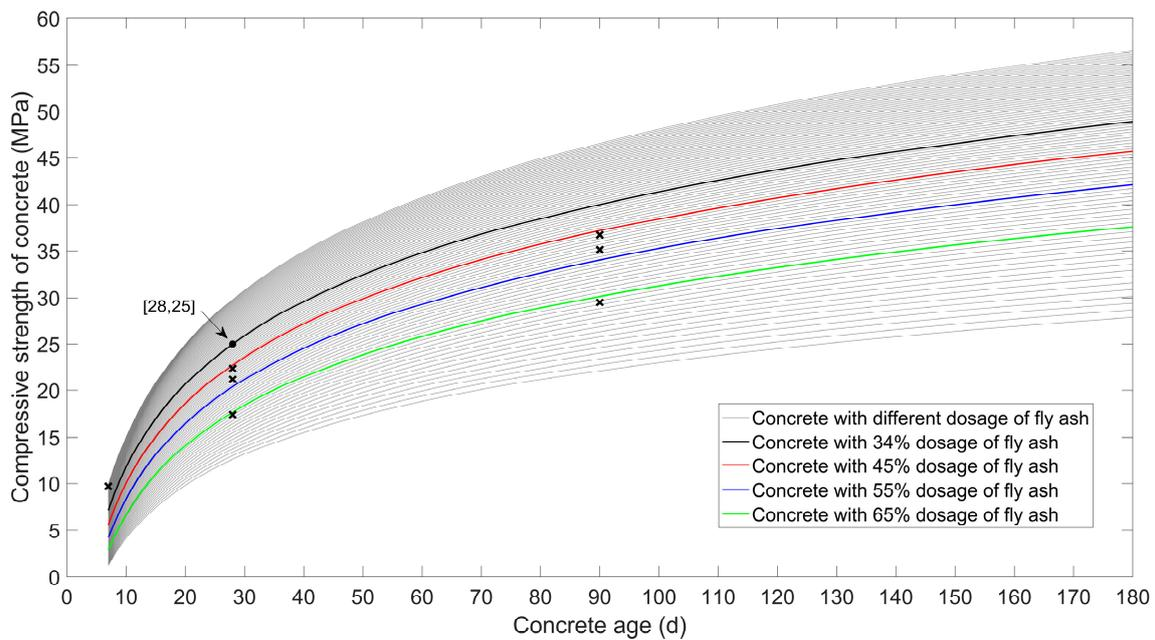
**Figure 9.** The relationship between the concrete’s age and compressive strength with 1% interval of the fly ash’s dosage. Black cross marks are tested value.
