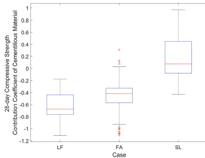
Figure 5. The 28-day compressive strength contribution coefficient of each cementitious material.
