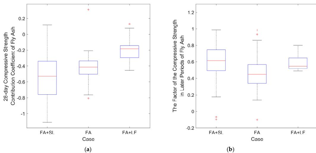
Figure 8. The 28-day compressive strength contribution coefficient of fly ash (a) and the factor of the compressive strength in later period of fly ash (b).
