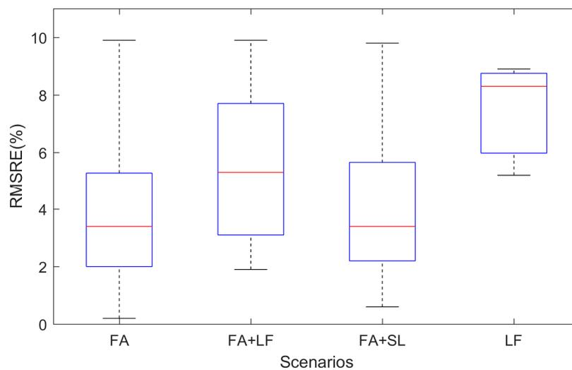
**Figure 4.** The root mean squared relative error of each kind of concrete. FA: concrete with fly ash; FA + LF: concrete with fly ash and limestone flour; FA + SL: concrete with fly ash and slag, and LF: concrete with limestone.
