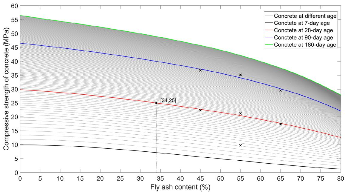
**Figure 10.** The relationship between fly ash content and compressive strength of concrete day-by-day. Black cross marks are tested value.
