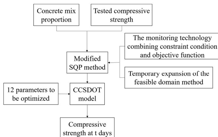
**Figure 2.** Overview of the model and methodology. SQP: sequence quadratic programming; CCSDOT: concrete compressive strength development over time.
