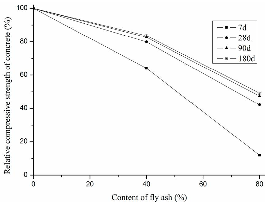
**Figure 11.** The relationship between the content of fly ash and the relative compressive strength of concrete.
