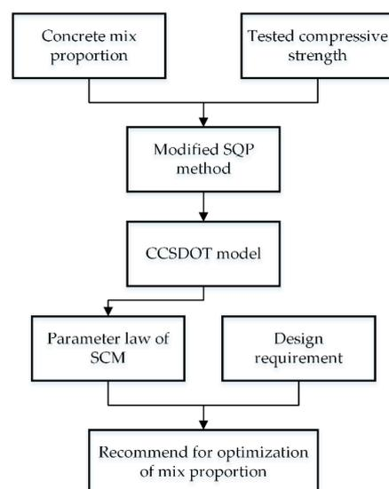
**Figure 1.** Overview of this study. CCSDOT: concrete compressive strength development over time; SQP: sequence quadratic programming; SCM: supplementary cementitious material.
