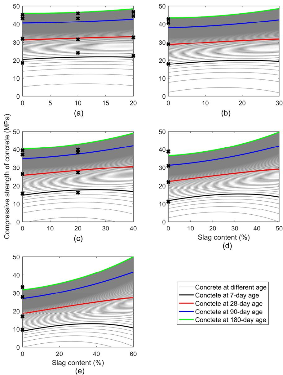
**Figure 12.** Comparison of concrete compressive strength with different doses of supplementary cementitious materials (slag and fly ash) at different ages day by day. The content of supplementary cementitious materials is 20% in (a), 30% in (b), 40% in (c), 50% in (d) and 60% in (e). Black cross marks are tested value.
