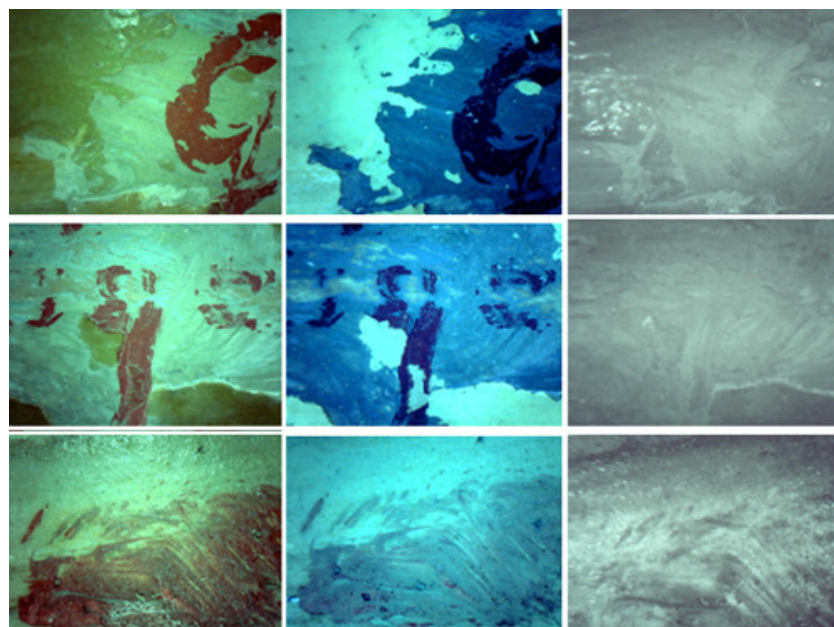
Figure 8. Analysis in the three reflected lights: white-green (550 nm), UV (365 nm), and IR (850 nm) of some areas with signature characters in Figure 7 and of other area where false writing is suspected.
