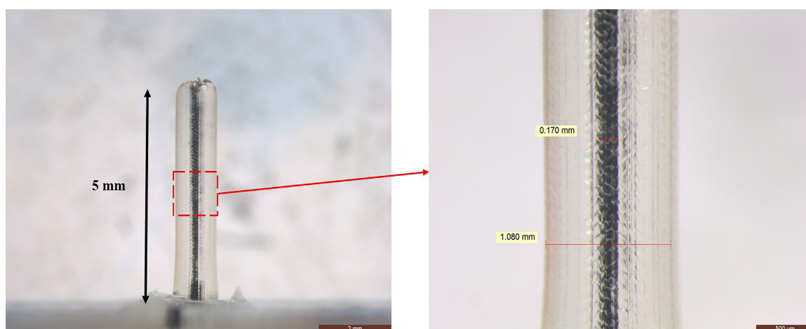
Figure 8. Dimension clarification and magnified view of successfully printed hollow connector.
