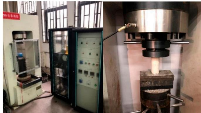
Figure 5. Uniaxial compression experiment apparatus.
