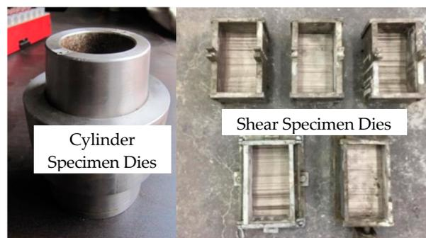
**Figure 3.** Cylinder and shear specimen dies.
