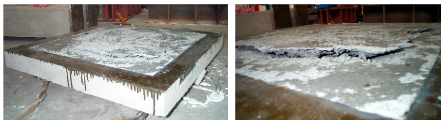
Figure 6. Punching shear failure on the tension surface of the specimen CSR1-C2-F2 after peeled off the CFRP laminates.
