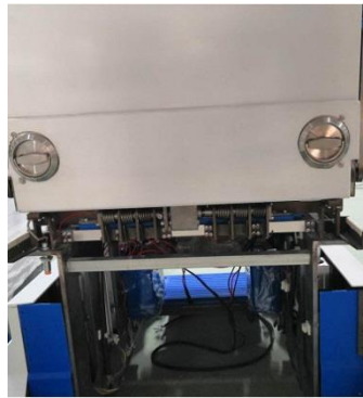
Figure 24. The driving device of folding mechanism.
