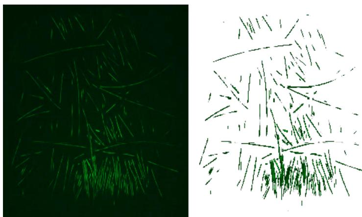
**Figure 6.** Example of threshold application on hair capacitive image. On the left the original frame, where acclimatized hair on bright green and air/bad contact on darker green shades. Right, the software output after a range threshold is applied to exclude pixels with bad contact before calculating water content.
