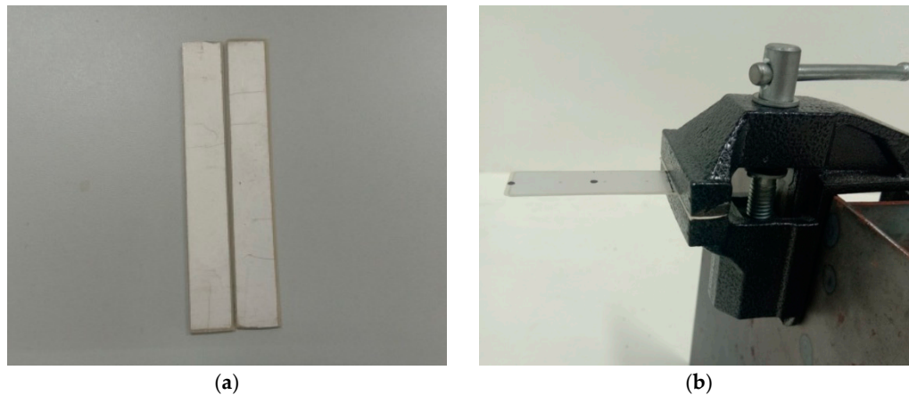
Figure 2. Scheme of the experimental specimens and piezoelectric cantilever beam: (a) PZT-5 piezoelectric ceramic specimens; (b) the piezoelectric cantilever beam.
