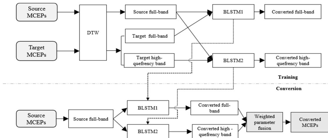
**Figure 2.** The flowchart of voice conversion with sub-band cepstrum conversion by BLSTMs. MCEPs: Mel-cepstral coefficients
