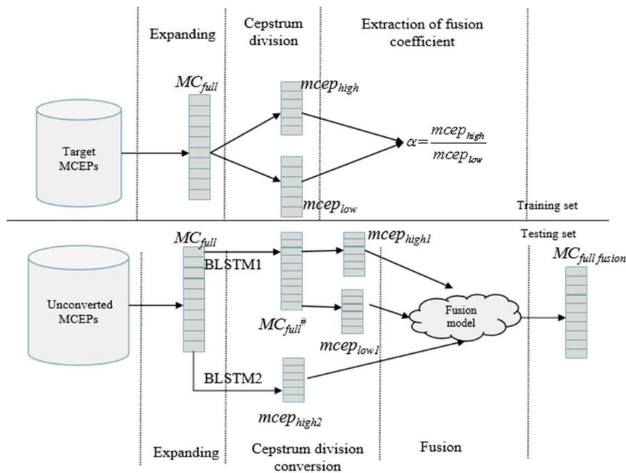
**Figure 3.** The diagram of the cepstrum-weighted fusion process, where the MC represents the full band MCEPs in different cases.
