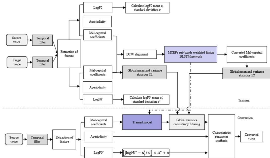
**Figure 1.** Voice conversion flow chart of sub-band cepstrum weighted fusion bidirectional long short-term memory (BLSTM). DTW: dynamic time warping.
