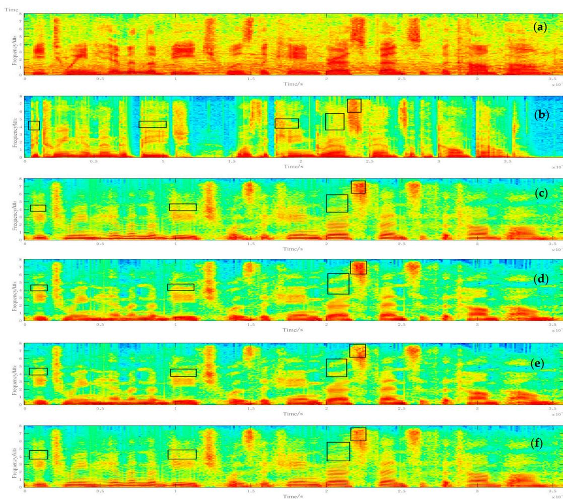
**Figure 6.** Spectrogram of the methods of voice conversion: (a) source voice with babble noise at 15 dB, (b) clean target voice, (c) BLSTM conversion, (d) the proposed method, (e) DIFFGMM conversion, and (f) GMM conversion.
