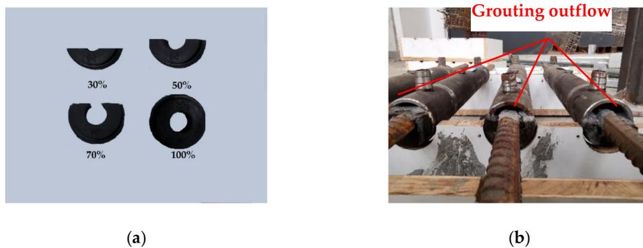
**Figure 2.** Settings of the grouting density: (a) cut rubber plugs; (b) sleeve locations where the grouting flowed out.
