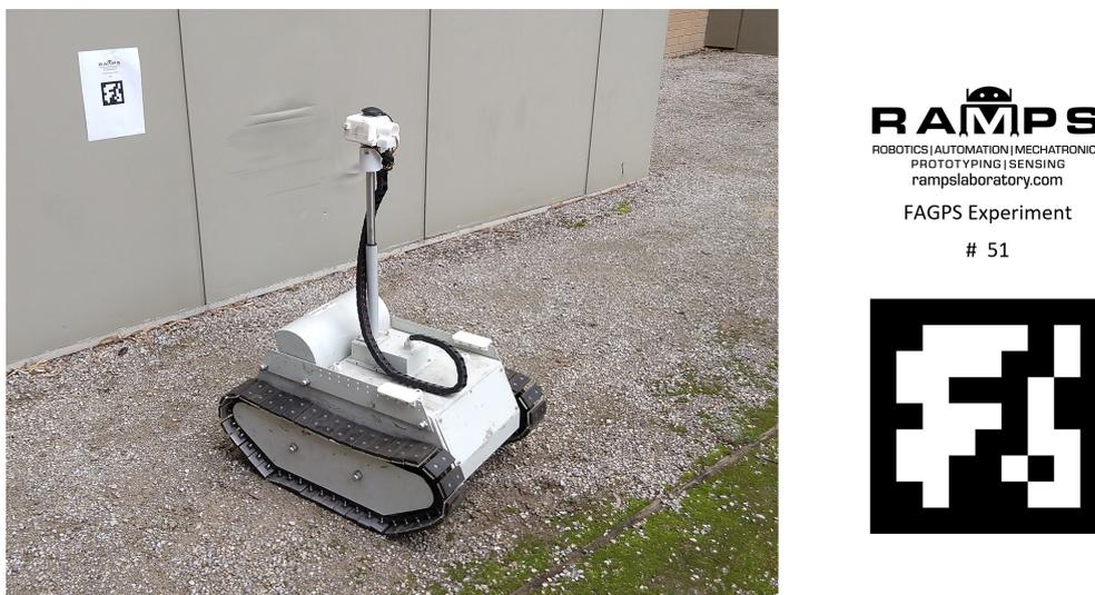
**Figure 1.** Robot performing visual pose estimation on a geolocated fiducial marker with fiducial shown on right.
