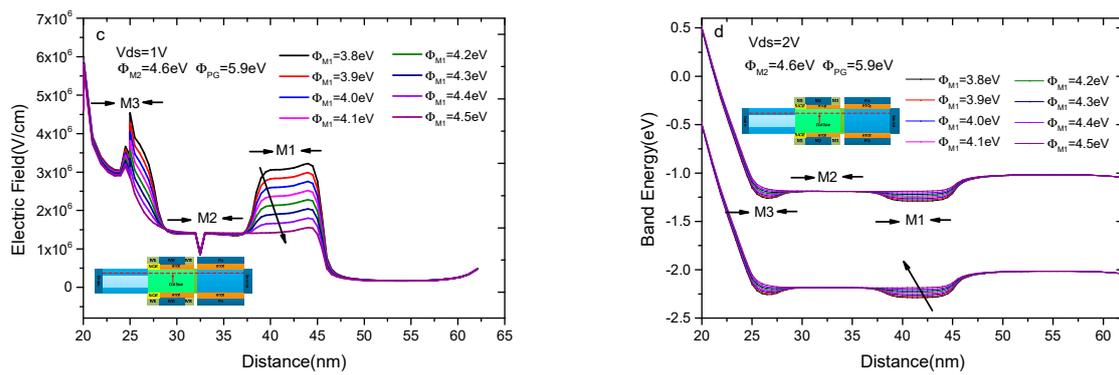
**Figure 9.** (a) Simulated log scale and linear scale transfer characteristics of DMMG-HJLTFET with different auxiliary gate work function ( $\Phi_{M1}$ ); (b) the potential distribution at the surface with different auxiliary gate work function ( $\Phi_{M1}$ ); (c) the distribution of electric field at the surface with different auxiliary gate work function ( $\Phi_{M1}$ ); (d) the variation of ON-state energy band with different auxiliary gate work function ( $\Phi_{M1}$ ).
