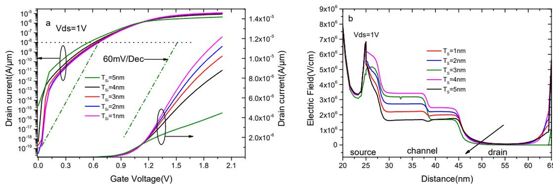
**Figure 10.** (a) Simulated log scale and linear scale transfer characteristics of DMMG-HJLTFET with different thickness of silicon ( $T_S$ ) in sandwich stack structure (GaAs/Si/GaAs); (b) the distribution of electric field at the surface with different thickness of silicon ( $T_S$ ) in sandwich stack structure (GaAs/Si/GaAs).
