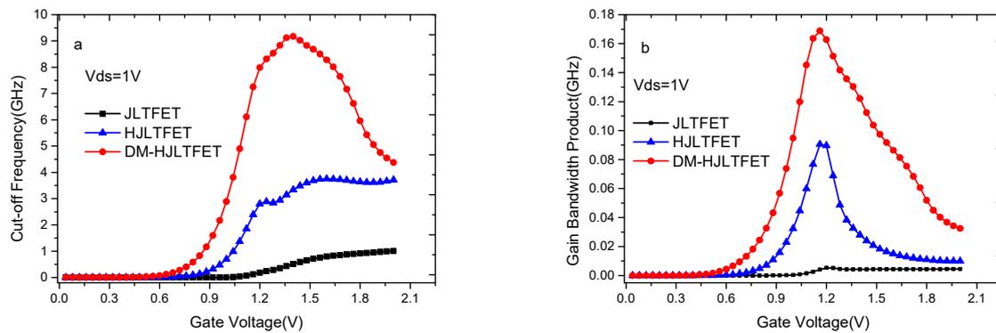
**Figure 12.** (a) The cut-off frequency ( $f_T$ ) characteristic curves of JLTFET, HJLTFET and DMMG-HJLTFET; (b) the gain bandwidth (GBW) characteristic curves of JLTFET, HJLTFET and DMMG-HJLTFET.
