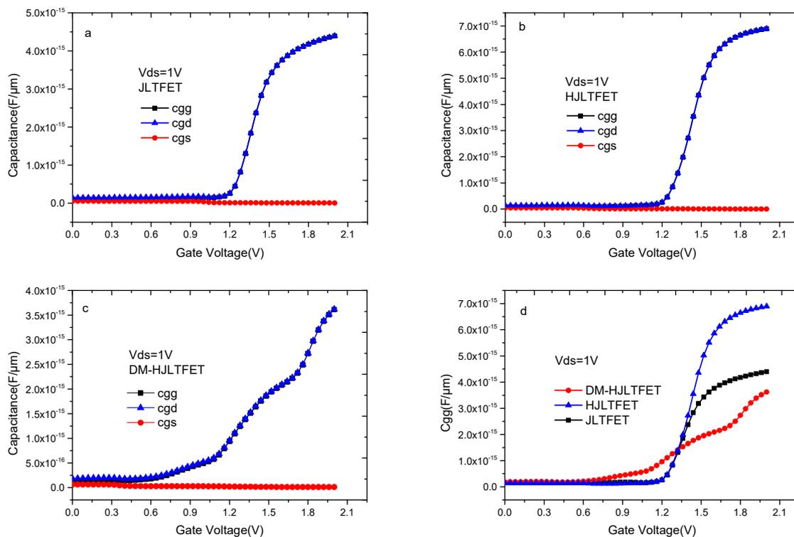
**Figure 11.** (a) Capacitance of JLTFET versus Vgs; (b) capacitance of HJLTFET versus Vgs; (c) capacitance of DMMG-HJLTFET versus Vgs; (d) comparison of Cgg (gate capacitance) of JLTFET, HJLTFET and DMMG-HJLTFET versus Vgs under Vds = 1.0 V.
