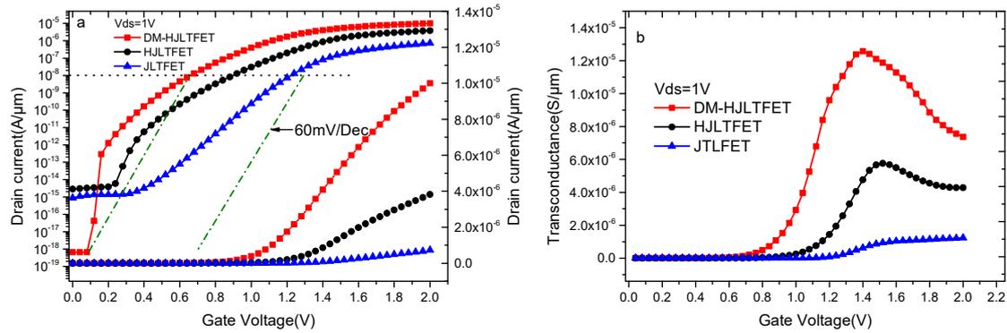
**Figure 4.** (a) The log scale and linear scale transfer characteristics of JLTFET, HJLTFET, and DMMG-HJLTFET; (b) transconductance of JLTFET, HJLTFET and DMMG-HJLTFET.
