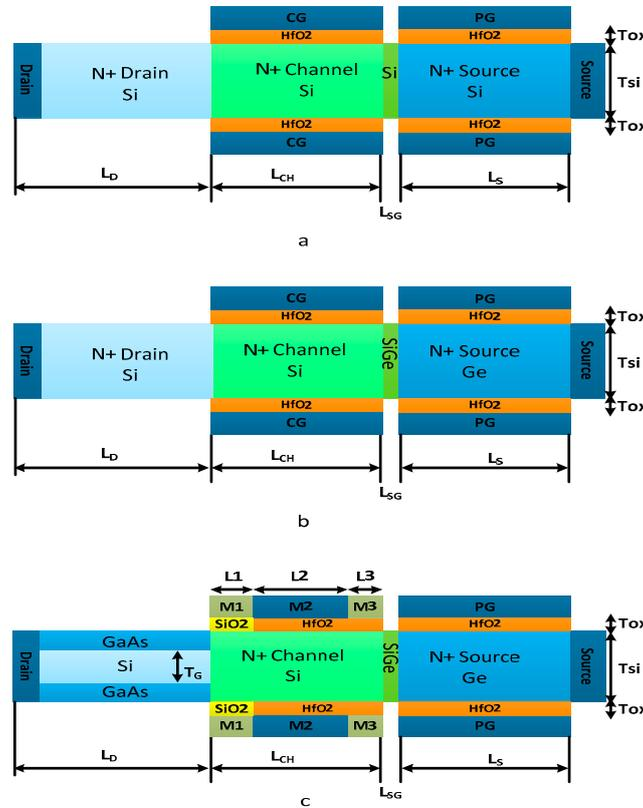
Figure 1. Cross-sectional view of (a) JLTFT; (b) HJLTFT; (c) DMMG-HJLTFT.
