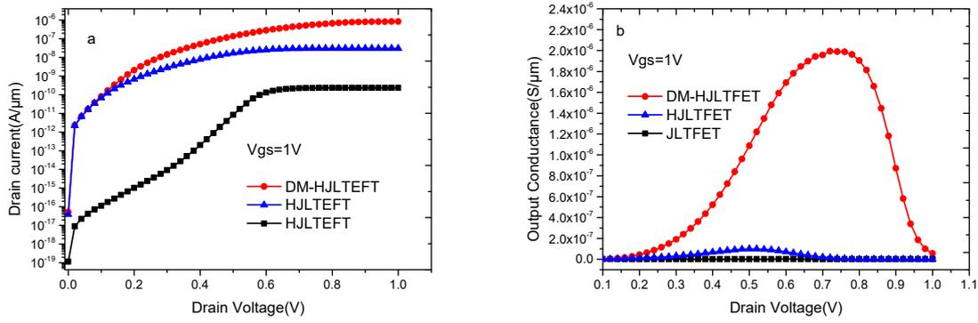
**Figure 5.** (a) Simulated output characteristics and (b) Simulated output transconductance of JLTfET, HJLTfET and DMMG-HJLTfET at  $V_{gs} = 1$  V.
