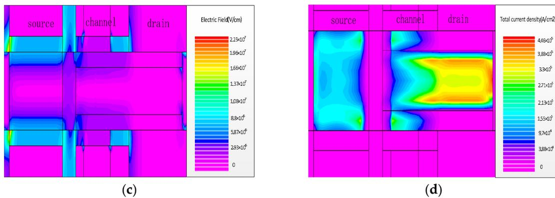
**Figure 2.** (a) Nonlocal band to band tunneling (BTBT) rate of electron; (b) nonlocal band to band tunneling (BTBT) rate of hole; (c) electric field distribution in DMMG-HJLTFET; (d) total current density of DMMG-HJLTFET.
