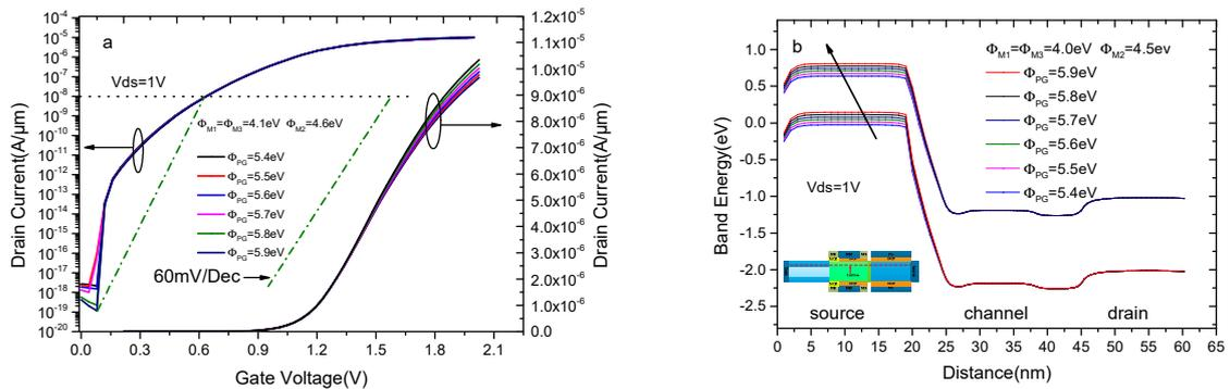
**Figure 7.** (a) Simulated log scale and linear scale transfer characteristics of DMMG-HJLTFET with different polar gate work function ( $\Phi_{PG}$ ); (b) the variation of energy band with different polar gate work function ( $\Phi_{PG}$ ).
