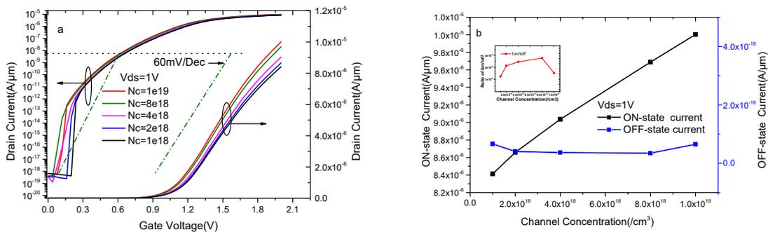
**Figure 6.** (a) Simulated log scale and linear scale transfer characteristics of DMMG-HJLTfET with different channel doping concentration; (b) ON-state current, OFF-state current and  $I_{on}/I_{off}$  at different channel doping concentration.
