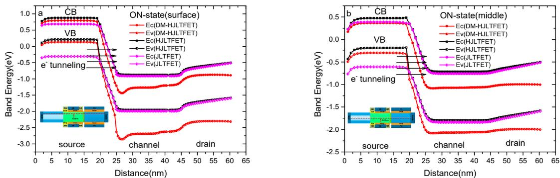
**Figure 3.** (a) The energy band diagram of JLTfET, HJLTFET and DMMG-HJLTFET at the device surface region; (b) The energy band diagram of DMMG-HJLTFET at the device middle region.
