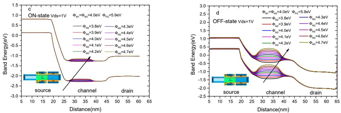
**Figure 8.** (a) Simulated log scale and linear scale transfer characteristics of DMMG-HJLTFET with different control gate work function ( $\Phi_{M2}$ ); (b) the distribution of electric field at the surface with different control gate work function ( $\Phi_{M2}$ ); (c) the variation of ON-state energy band with different control gate work function ( $\Phi_{M2}$ ); (d) the variation of OFF-state energy band with different control gate work function( $\Phi_{M2}$ ).
