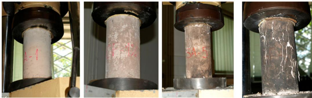
**Figure 7.** Compression testing to breaking point in test pieces without addition and with 1% CNFs, before and after fire testing.
