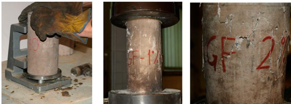
**Figure 3.** Capping of test pieces and compression testing to breaking point.
