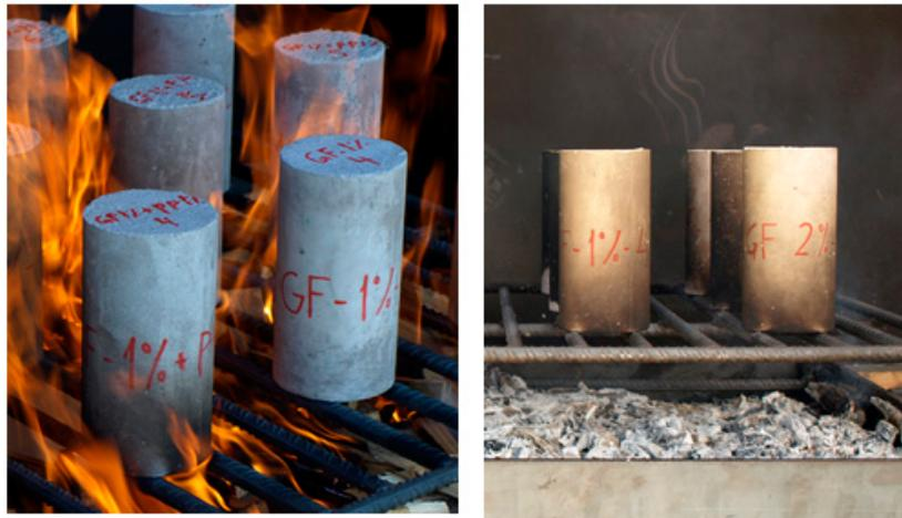
**Figure 2.** Fire test involving the entire surface of the test piece being directly exposed to the fire and taking measurements with an infrared thermometer.
