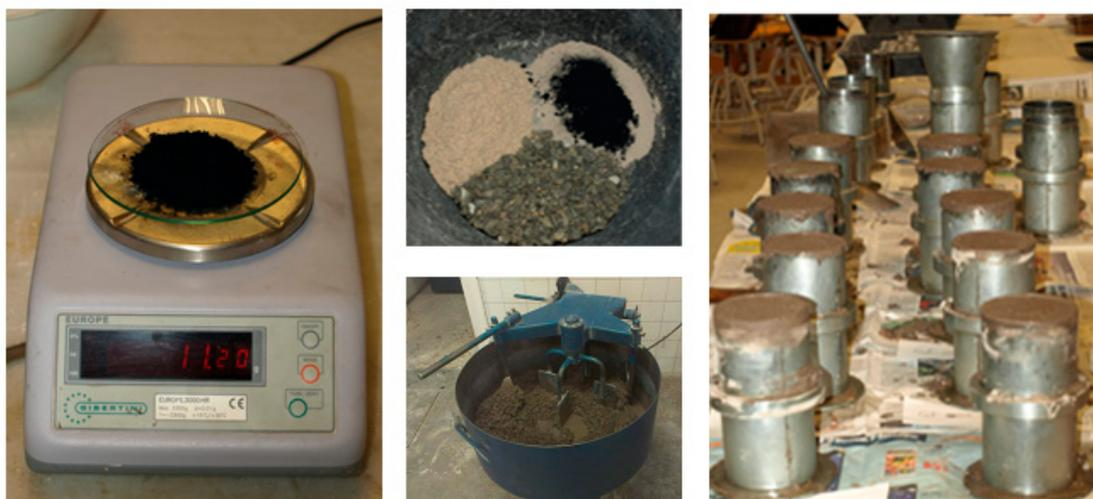
**Figure 1.** Process of manufacturing cylindrical test pieces with and without addition: dosage, standardization, mixing and molding.
