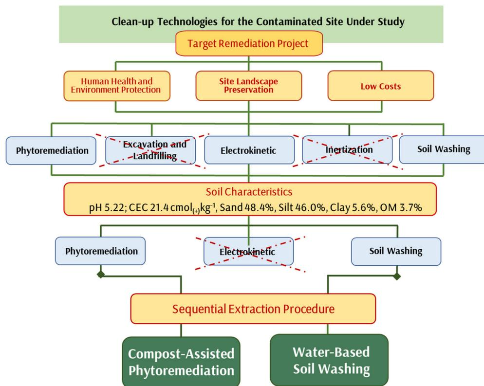
**Figure 1.** Scheme of technologies screening based on soil properties of the contaminated soil.
