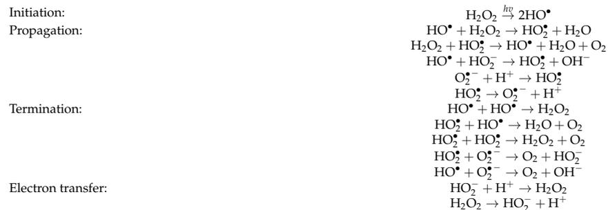
The degradation kinetics of UV/ $\text{H}_2\text{O}_2$  in the treatment of PVA-containing wastewater was first modeled by Hamad et al. (2018), where an overview of the degradation process is as follows:
