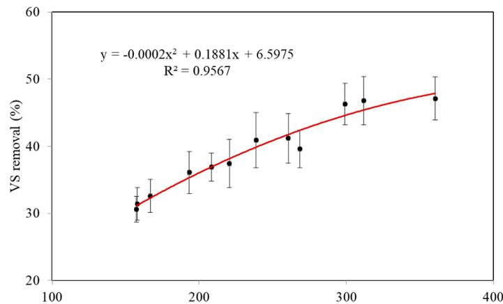
Figure 4. Correlation of biogas produced per g volatile solids (VS) and percentage of VS removal for all the experiments.
