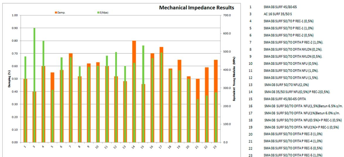
Figure 9. Mechanical impedance results for the 23 different mixtures.
