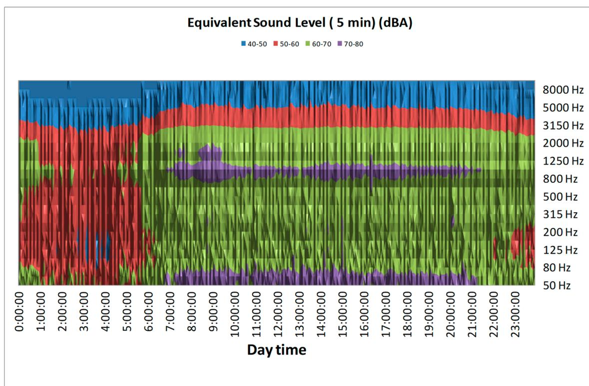
**Figure 2.** Frequency analysis of sound pressure levels at point 1 at the A-376 site.
