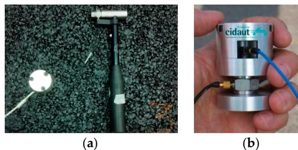
**Figure 6.** (a) Mechanical impedance setup. (b) Impedancimeter.
