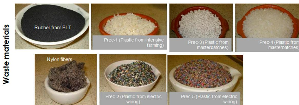
**Figure 5.** Materials used for generating the additives for asphalt mixes.
