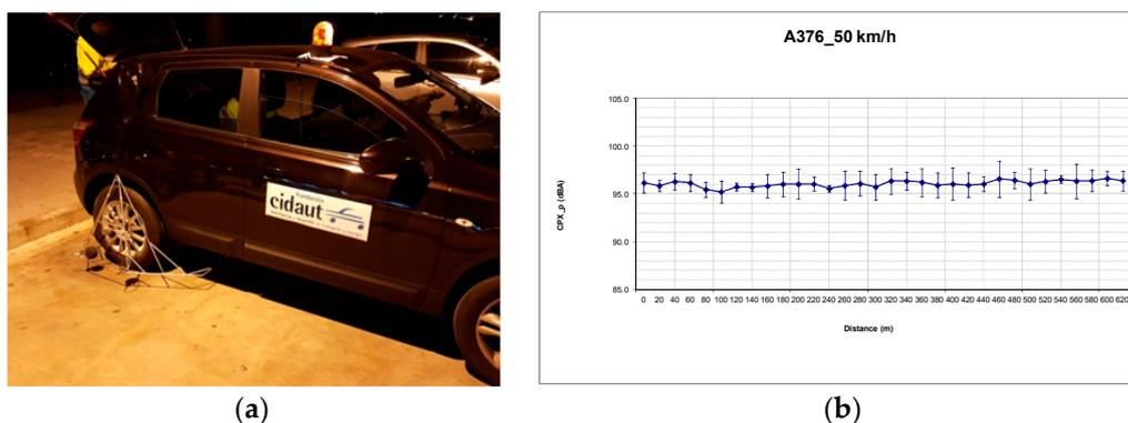
**Figure 4.** (a) Image of the self-propelled vehicle used for the close proximity (CPX) measurements. (b) Results of  $CPX\_p$  at the A-376 site at 50 km/h.
