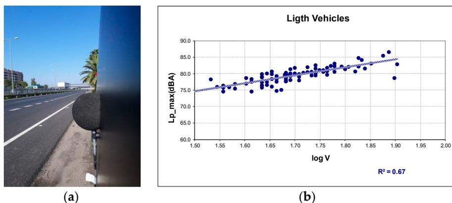
**Figure 3.** (a) Image of the statistical pass by noise test (SPB) test at A-376 site. (b) Results of  $Lp\_max$  at A-8058 site for the regression analysis.
