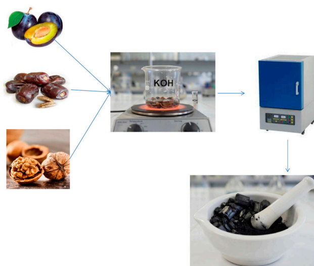
Figure 1. Synthesis procedure of activated carbons obtained from plum stones, date stones and walnut shells.
