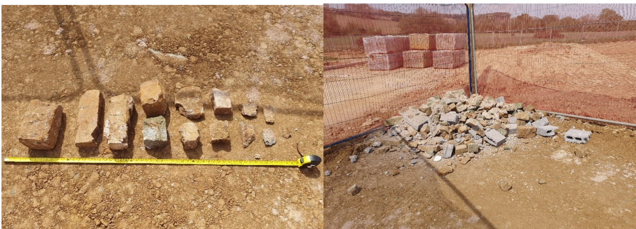
Figure 5. Photographs taken during the study of brick and block waste that was transferred from the tipping skip to the compound area for recording, and ironstone brick waste (used as a facing material) being measured for input into the Construction Waste Indicative Cost (CWIC) Calculator.
