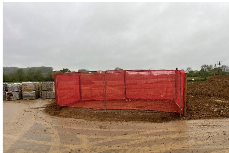
Figure 4. Photograph of the study compound set-up on site, designed to facilitate the storage and measurement of waste during the controlled study.
