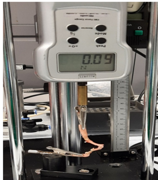
Figure 2. A sealing seam was pulled vertically upwards apart. Structural failure occurred exclusively within the sealing zone; there were no cracks or slippage around the clamps. The digital display remains at maximum peel pressure (own photo).
