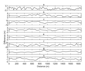
**Figure 4.** Plots of height differences between profiles extracted from the investigated DEMs minus the leveling along the runway's centerline: (**a**) aerial photogrammetry DEM; (**b**) ASTER; (**c**) AW3D30; (**d**) SRTM-1"; (**e**) SRTM-3"; (**f**) SRTM-X; (**g**) TanDEM; (**h**) WorldDEM<sup>TM</sup>. Note the different vertical scales on the vertical axes.
