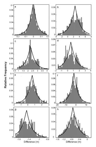
**Figure 5.** Histograms of the differences between the investigated DEMs and leveling: (**a**) aerial photogrammetry DEM; (**b**) ASTER; (**c**) AW3D30; (**d**) SRTM-1"; (**e**) SRTM-3"; (**f**) SRTM-X; (**g**) TanDEM; (**h**) WorldDEM<sup>TM</sup>. A theoretical Laplace probability density function is also shown. The function parameters were estimated using the experimental data. They are shown in Table 4.
