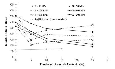
**Figure 8.** Deviator stress at failure versus rubber waste content for (RCR) mixtures and for the clay and clay-crumb mixtures (based on this study and Tajdini et al.'s tests [31]).
