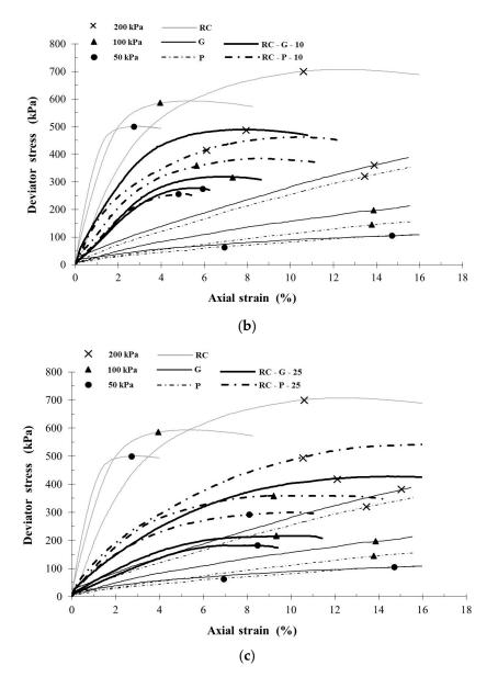
**Figure 6.** Deviator stress versus axial strain for pure red clay, powder and granulate, and for RCR mixtures, under confining pressure 50, 100, and 200 kPa: (**a**) 5% addition of (P) or (G), (**b**) 10% addition of (P) or (G), and (**c**) 25% addition of (P) or (G).
