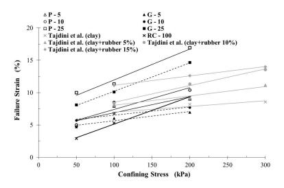
**Figure 9.** Strain at failure versus confining stress for (RCR) mixtures and for the clay and clay-crumb mixtures (based on this study and Tajdini et al.'s tests [31]).
