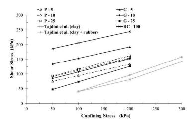
**Figure 7.** Shear stress versus confining stress for (RCR) mixtures and for the clay and clay-crumb mixtures (based on this study and Tajdini et al.'s tests [31]).
