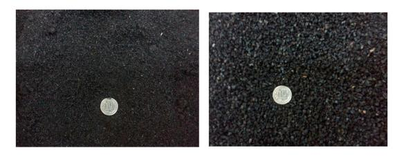
(a) (b) Figure 1. Rubber waste: (a) powder (P) 0–1 mm, (b) granulate (G) 1–5 mm.
