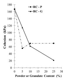
Figure 5. Variation of the cohesion with the rubber waste content.
