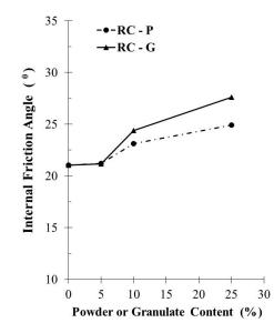
Figure 4. Variation of the angle of internal friction with the rubber waste content.
