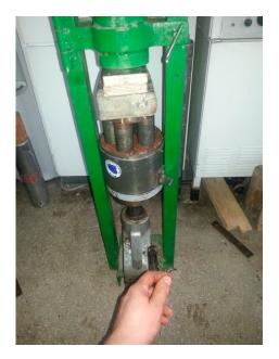
Figure 2. Preparation of specimens from the Red Clay-Rubber (RCR) mixture.
