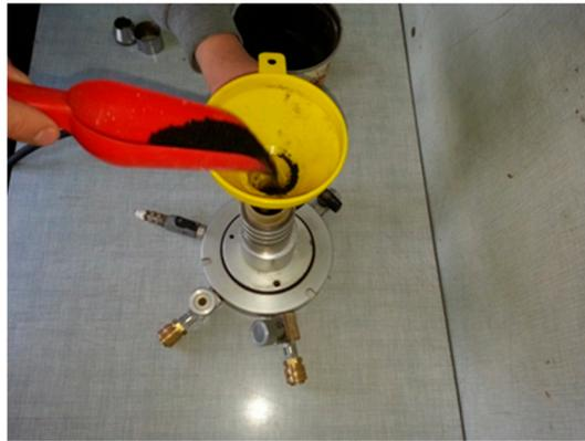
Figure 3. Preparation of specimens from the pure powder or granulate.
