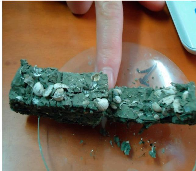
Figure 8. Photographs of a dry direct shear test (DST) specimen from the top layer rich in shell fragments.
