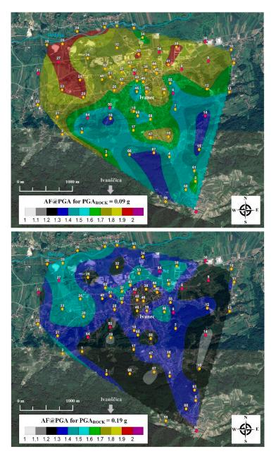
**Figure 14.** Up: Map of site response amplification factor at surface peak ground acceleration *PGA* for input  $PGA_{ROCK} = 0.09$  g (95yrp). Bottom: Map of site response amplification factor at surface peak ground acceleration *PGA* for input *PGA<sub>ROCK</sub>* = 0.19 g (475 yrp).
