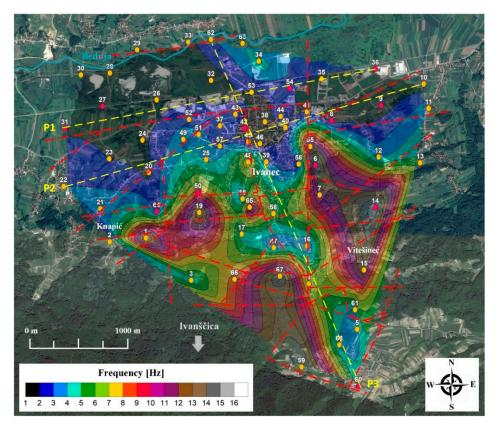
**Figure 6.** Map of the fundamental HVSR soil frequencies obtained for the City of Ivanec with marked faults (red dashed lines) based on geological map (Figure 3). Yellow circles indicate microtremor measurements and red geophysical measurements. Extrapolated HVSR amplitude-frequency contours vs. distance profiles marked with yellow dashed lines will be shown in Figure 10.
