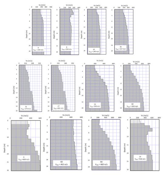
**Figure 7.** 1-D shear wave velocity profiles derived from MASW measurements with estimated values of  $V_{S30}$ . Note that profiles for sites 27 and 31 didn't reach depth of 30 m as other sites due to very low surface shear wave velocity.
