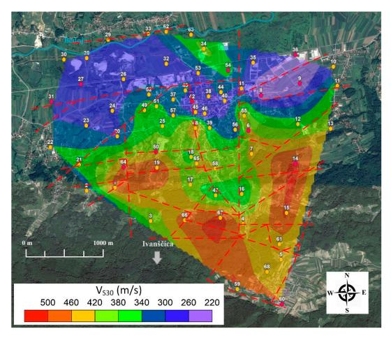
**Figure 11.** Map of  $V_{530}$  distribution for the City of Ivanec. Red circles indicate location of geophysical measurements and yellow microtremor measurements. According to Eurocode 8 soil classification [30], city area can be divided into soil classes B (360–800 m/s) and C (180–360 m/s).
