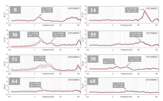
**Figure 5.** Selected examples of HVSR curves showing clear (8, 14), broad (51, 55) and multiple peaks (30, 38) with examples of flat HVSR curves that show small peak (64, 68). The average HVSR plot is represented by a thick red line and fundamental frequencies are marked with grey arrow. Black thin lines indicate the 95 % confidence interval of the HVSR.
