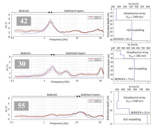
**Figure 8.** Examples of H/V forward modelling routine: Left: Observed H/V spectra (red) fitted with theoretical HVSR curve for representative soil model shown in right figures. Right: Values of  $V_{S30}$  estimated from geophysical data and H/V forward modelling.
