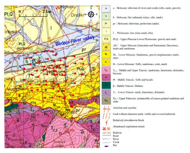
**Figure 3.** Geological map of the City of Ivanec area between Bednja River valley and Mt. Ivanščica (highest point Ivanščica at 1060 m elevation). Red circles indicate microtremor measurement locations [36].
