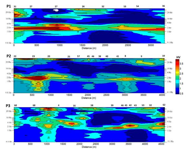
**Figure 10.** Extrapolated HVSR amplitude-frequency contours vs. distance profiles (marked with yellow dashed lines in Figures 6 and 9). Microtremor measurement locations are marked above figure.
