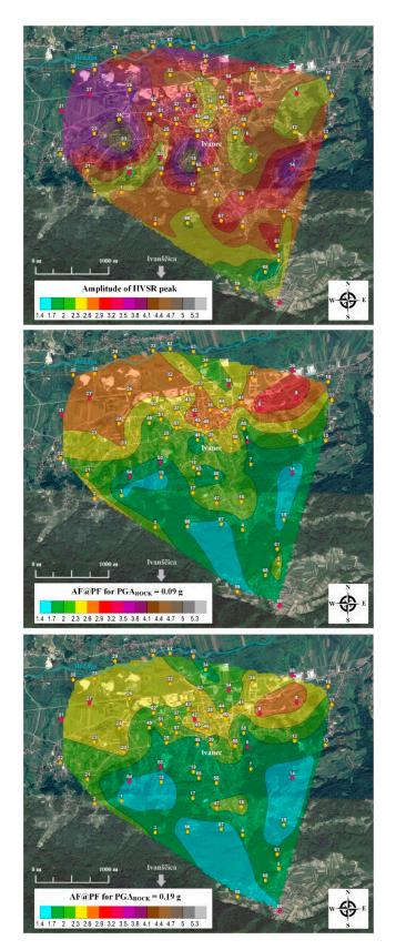
**Figure 13.** Up: Map of the amplitude of HVSR peak at fundamental HVSR frequency. Middle: Map of site response amplification factor at predominant frequency for input  $PGA_{ROCK} = 0.09$  g (95yrp). Bottom: Map of site response amplification factor at predominant frequency for input  $PGA_{ROCK} = 0.19$  g (475yrp). The same colour scale for the amplification is used in all three cases.
