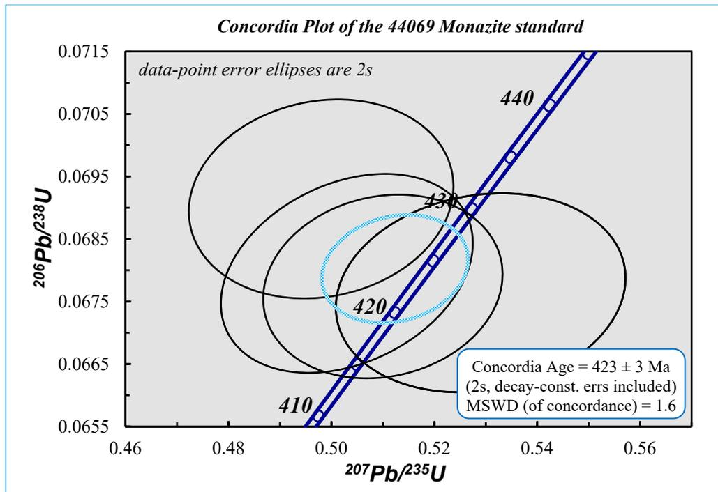
**Figure S1.** Results of U-Pb geochronology of the 44069 monazite standard that was used to check the accuracy of the data ( $424.9 \pm 0.4$  Ma; [37]).
