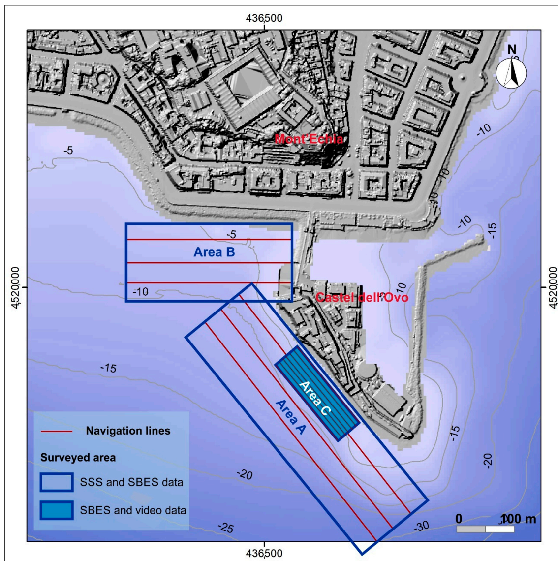
Figure 6. Map of the navigation carried out during the indirect survey. The shaded relief in the figure has been calculated from the digital surface model (DSM, with a grid 1 \times 1 m), provided by the Municipality of Naples.
