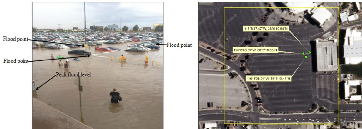
**Figure 10.** Imagery used for model calibration showing the location of some of the known flood points and the peak depth location at the inlet where watermark was still intact after flooding (on the left) verified through a field visit, and the exact geographic location of the points recorded via field visit with a GPS (on the right). Courtesy of Rebel Yell, University of Nevada Las Vegas.
