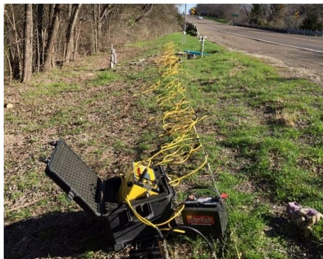
Figure 3. Resistivity set up at slope of SH 342.
