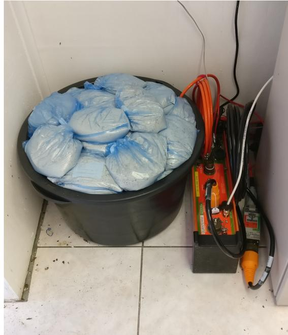
**Figure 9.** Seismic installation at station SABV. The seismometer rests on the tiles on the concrete floor and is completely surrounded by dry sand in a quasi-flexible container. Next to the sensor is the datalogger.
