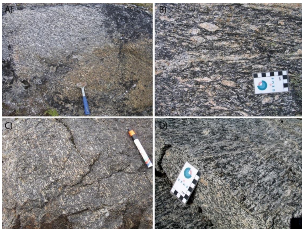
Figure 2. Field images illustrating characteristic textures from the Ilivertalik Intrusive Complex. (A) Out-crop relation between sample 484645 (upper left part of image) and sample 484644 lower right part of image) the brown alteration colour is characteristic of pyroxene bearing units. The sharp crosscutting the S-L textures in the granite, suggest that retrogression into amphibolite facies occurred after ductile deformation overprinting. (B) Characteristic feldspar clastic granite unit. (C) Texture of a dioritic unit (equivalent to sample 508204). (D) Lineated granodiorite (equivalent to sample 468689).
