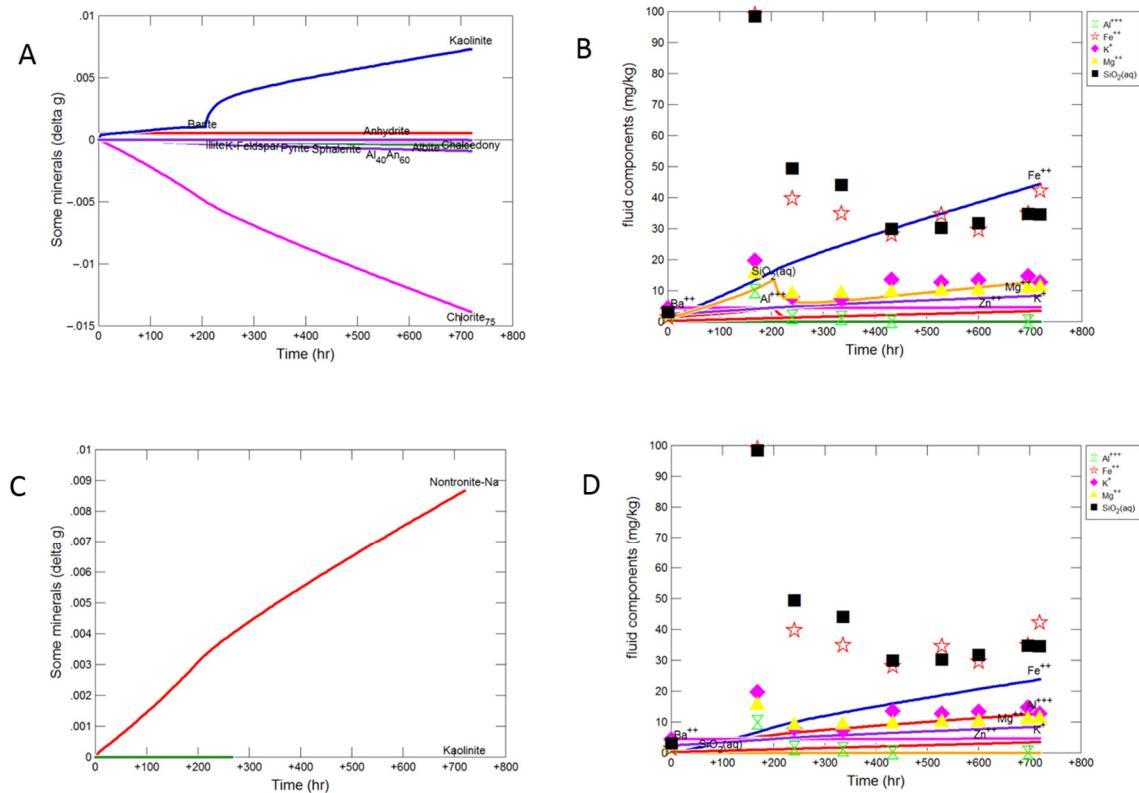
**Figure S8.** Additional experimental models (lines) and experimental data (symbols) for calcite cemented cap-rock reaction: A) and B) change in minor minerals mass (grams) and water chemistry without kaolinite and goethite script file modification, C) and D) smectite and kaolinite mineral precipitation mass (grams), and water chemistry when smectite precipitation was unsuppressed.
