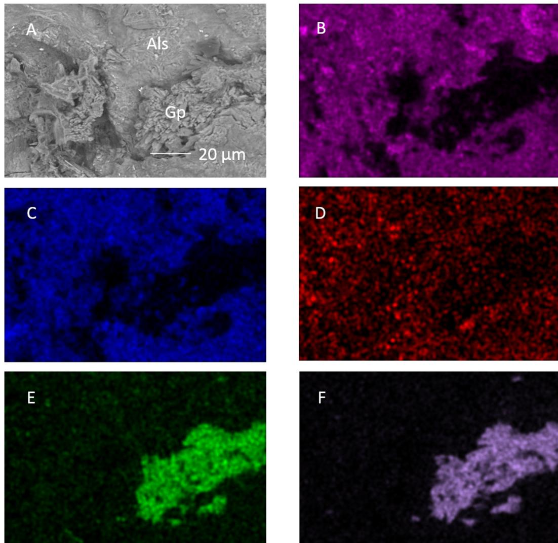
**Figure S1.** Scanning Electron microscope (SEM) image and EDS element maps after reaction showing precipitated gypsum (Gp), Aluminosilicate layer (Als) and skeletal clay (indicated with an arrow). Colours in B - F indicate a relatively stronger element concentration. A) SEM image, B) Pink = Si, C) Blue = Al, D) Red = Fe, E) Green = Ca, F) Purple = S.
