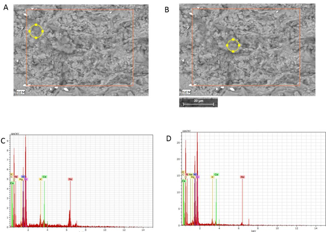
**Figure S2.** SEM and EDS spectra of corroded chlorite surface after reaction. A) SEM image of corroded chlorite surface, B) Circle marks a precipitated amorphous material. C) EDS spectrum of corroded chlorite surface marked in A, D) EDS spectrum of precipitated amorphous material marked in B.
