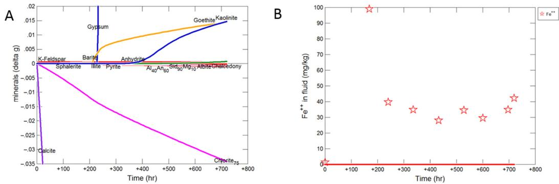
**Figure S7.** Experimental models (lines) and experimental data (symbols) for calcite cemented cap-rock reaction: A) Magnified view of minor mineral mass (grams) dissolving and precipitating in the final experimental model. B) Dissolved Fe when hematite precipitation was unsuppressed.
