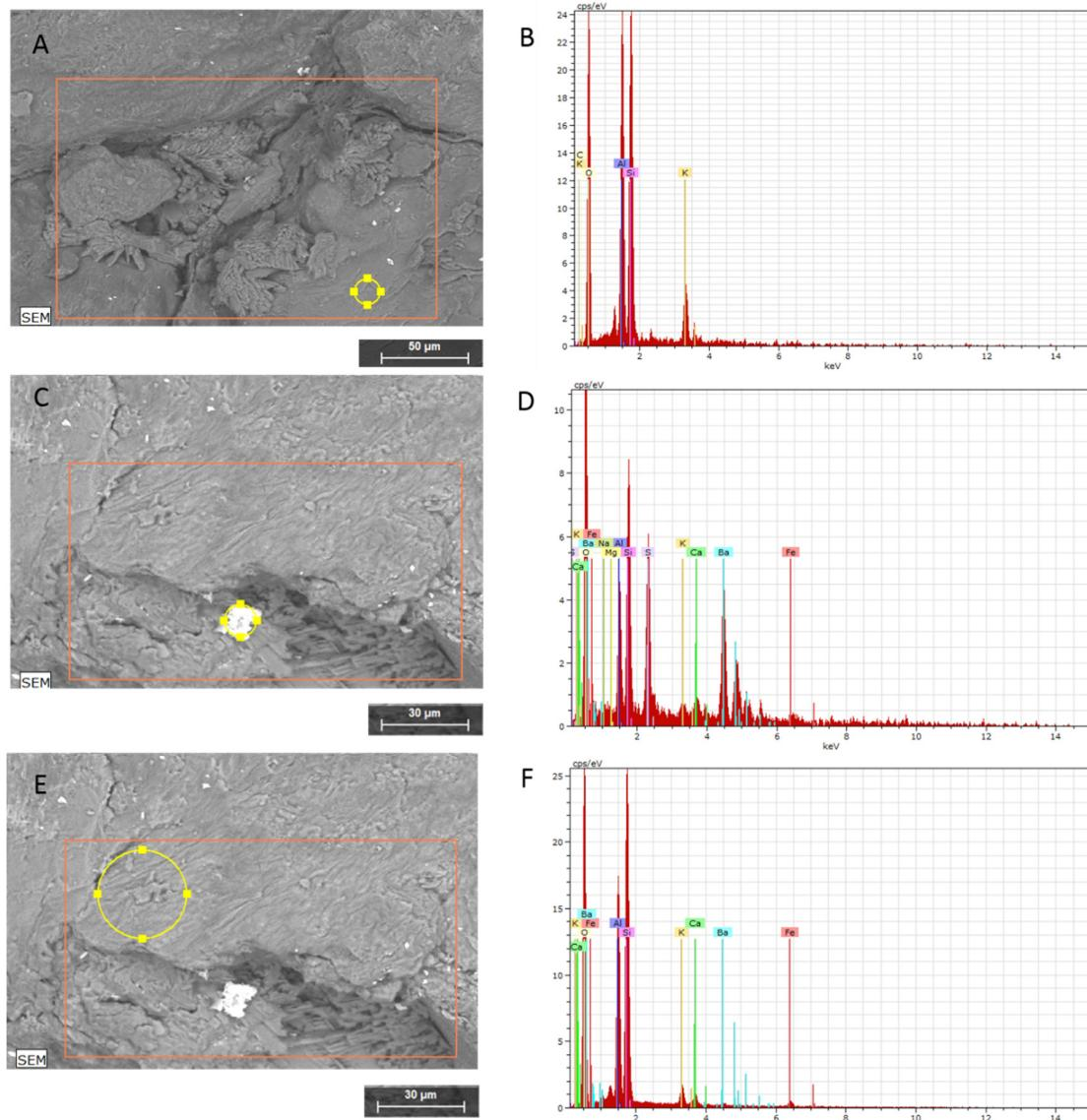
**Figure S3.** SEM images and EDS spectra of the inside surface of the block after reaction. A) Gypsum growing in created pore, B) EDS spectrum of marked K-feldspar grain in A, C) Precipitated barite, D) EDS spectrum of barite in C, E) precipitated aluminosilicate material, F) EDS spectrum of precipitate marked in E with a Si:Al ratio similar to kaolinite.
