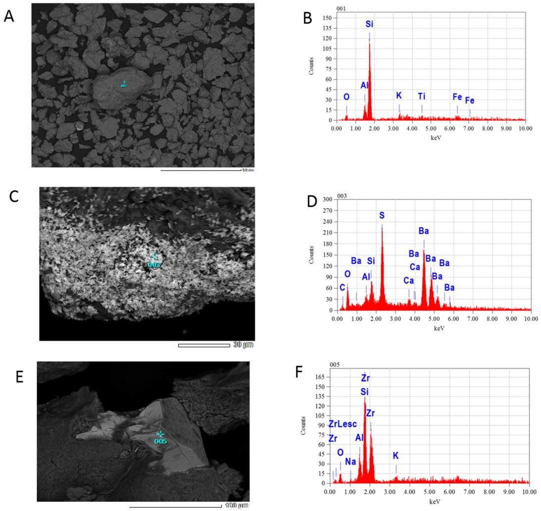
**Figure S6.** SEM images and EDS spectra of dis-aggregated grains after reaction recovered from the reactor: A) and B) Framework grains covered in Fe-oxide or aluminosilicate coatings, C) and D) Precipitated bright barite crystals, E) and F) zircon with amorphous precipitated material coating surrounding grains.
