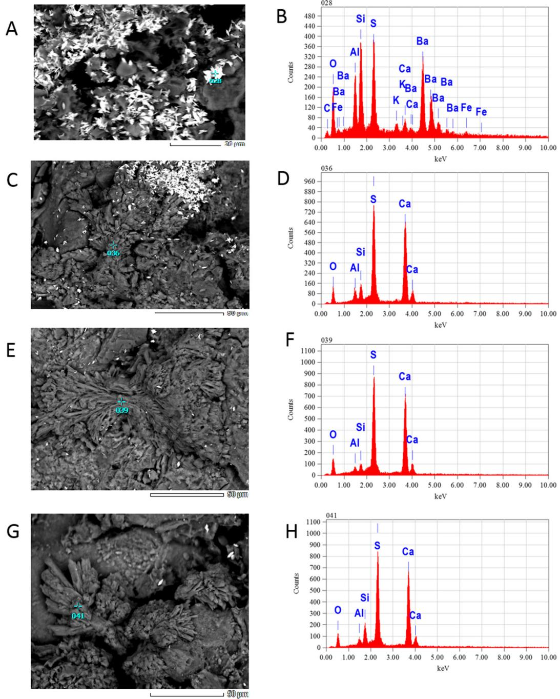
**Figure S5.** SEM images and EDS spectra of precipitated material after reaction: A) and B) Bright barite crystals precipitated on gypsum, C) to H) Gypsum growing from the pore space created by calcite dissolution.
