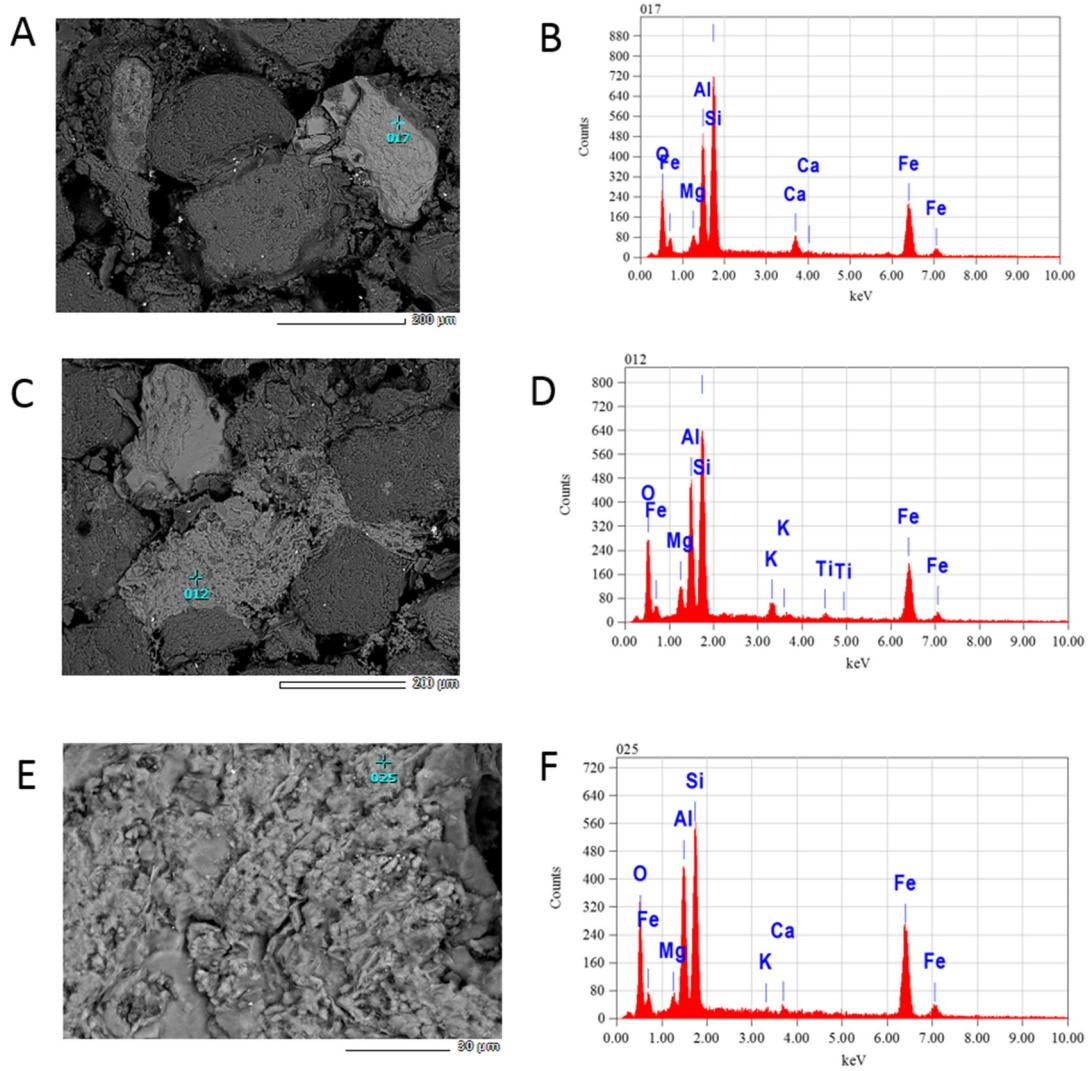
**Figure S4.** SEM images and EDS spectra of the exposed block surface after reaction. A) and B) garnet grain appears unaltered, C and D) mica appears unaltered, E and F) chlorite.
