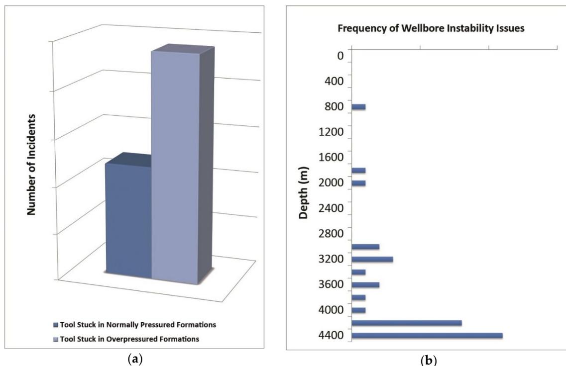
**Figure 8.** (a) Statistics of stuck tool (pipe, logging tools and bottom hole assemblies) events in some of the wells of the Abadan Plain Basin. (b) Frequency of wellbore instability issues in the Abadan Plain Basin. The majority of incidents occurred in the overpressured formations.
