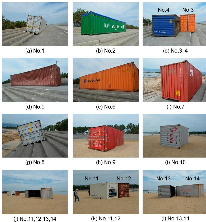
**Figure 10.** Photographs of the displaced containers. The numbers correspond to the identification numbers of each container shown in Table 3.
