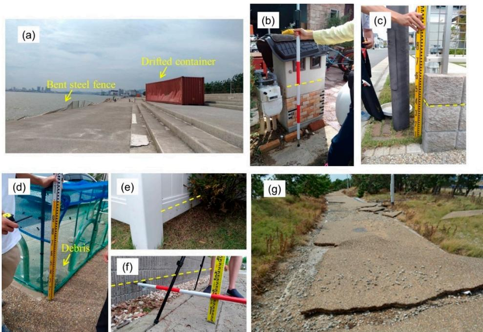
**Figure 8.** Photographs taken by the authors at Suzukaze town. (a) Damaged steel barrier and drifted shipment container at the embankment; (b–f) Survey Points S1–S5, respectively (watermark is highlighted with a yellow dashed line); (g) Eroded pedestrian road near the coastal embankment.
