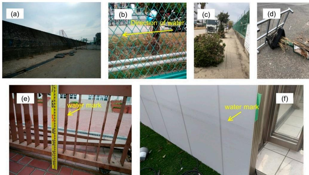
**Figure 7.** Photographs taken by the authors at Fukaeahama town. (a) Coastal dike at Fukaeahama town, (b) Survey Point F1 indicates that the direction of debris was towards the inland, (c–d) Presence of debris at Fukaeahama town, (e) Survey Point F2 (watermark at school gate), (f) Survey Point F3 (watermark at a model house).
