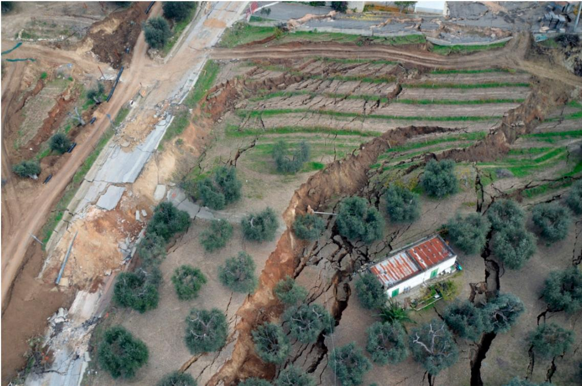
**Figure 10.** The picture (UAV image) shows clear and spectacular examples of decompression and graben structures developed by the landslide with the destruction of a road and a building.
