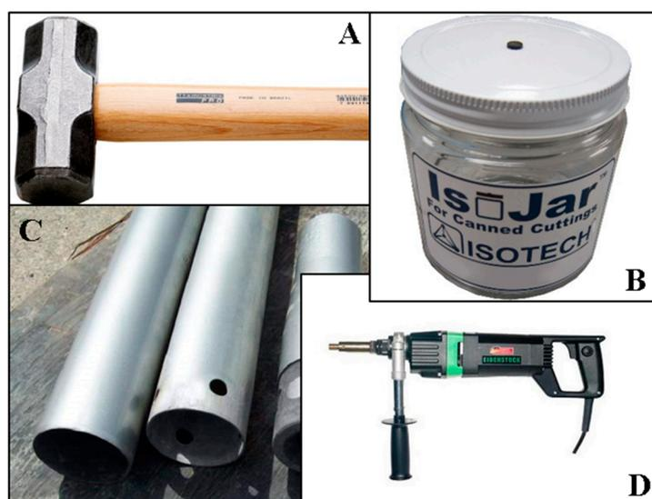
**Figure 4.** (A) Hammer; (B) IsoJar<sup>®</sup>, by Isotech (Weatherford International, Houston, TX, USA); (C) Tubes used for soil sampling; (D) Drilling machine used for deeper sampling.
