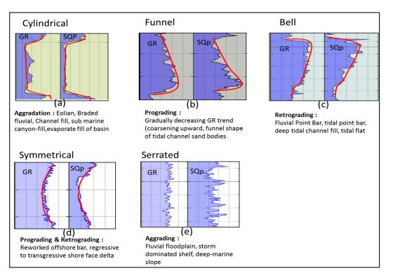
**Figure 3.** Facies identification in the gamma ray and *SQp*, the values of GR and *SQp* increase to the right. (a) Aggradation; (b) Prograding; (c) Retrograding; (d) Prograding & Retrograding; and, (e) Aggrading.
