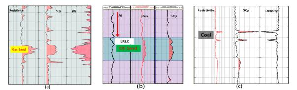
**Figure 4.** The responses of Resistivity and *SQs* logs in different environment: (**a**) Gas sand reservoir; (**b**) Low Resistivity Low Contrast (LRLC)-oil sand; and, (**c**) coal layer.
