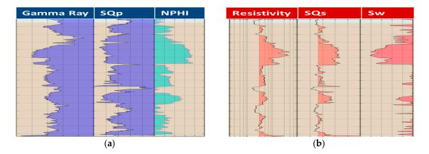
**Figure 2.** (a) *SQp* response compared with the gamma ray and neutron porosity log; and (b) *SQs* response when compared with the resistivity and water saturation log.
