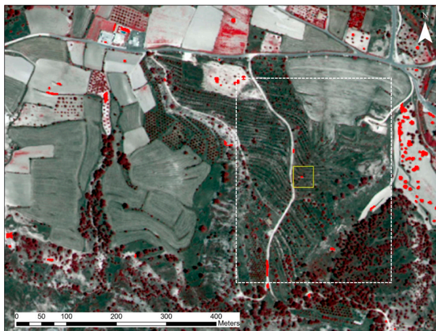
Figure 11. Object-oriented segmentation and classification of the WorldView-2 satellite image. The white rectangle shows the area of the necropolis under examination, while the yellow square shows the looting mark.
