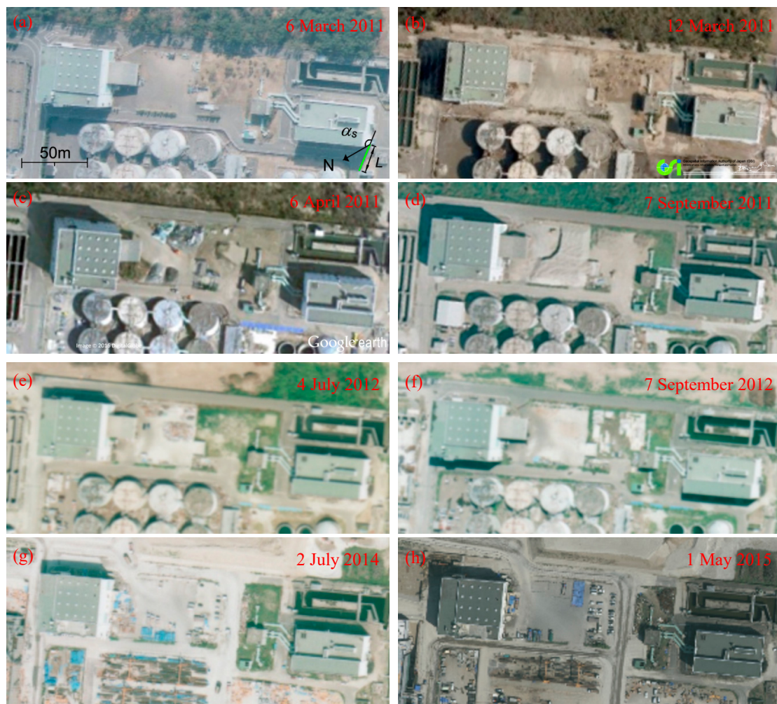
Figure 4. Measuring azimuth angle and length of shadow on aerial photographs and satellite images, (a–h) are the selected rectified images.
