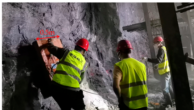
Figure 1. Image showing the field conditions for GPR-based irregular tunnel face.
