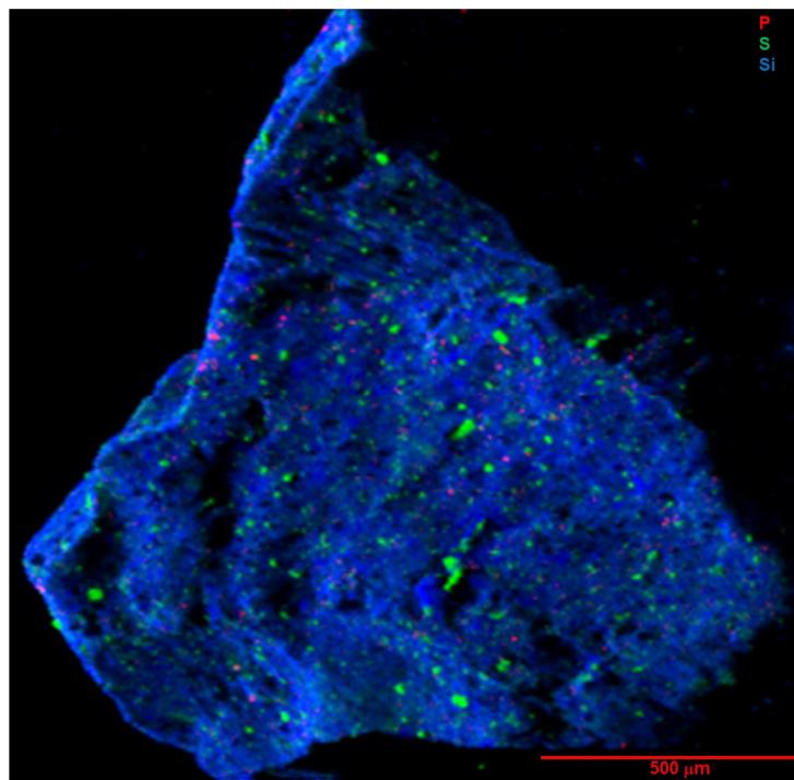
**Figure 8.** Tender-energy XRF map of whole-particle C0034, showing P, S, and Si as in Figure 7. Image was measured at the TES beamline with incident beam energy of 2.7 keV, beam focus size of 5  $\mu\text{m}$ , and 5  $\mu\text{m}$  pixel size.
