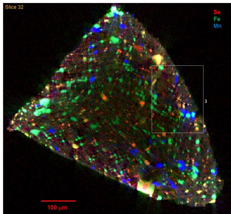
**Figure 3.** High-resolution tomographic slice number 32, voxel size  $2 \times 2 \times 1 \mu\text{m}$  and showing Se (red), Fe (green), and Mn (blue). Outlined area 3 is shown in more detail in Figure 5.
