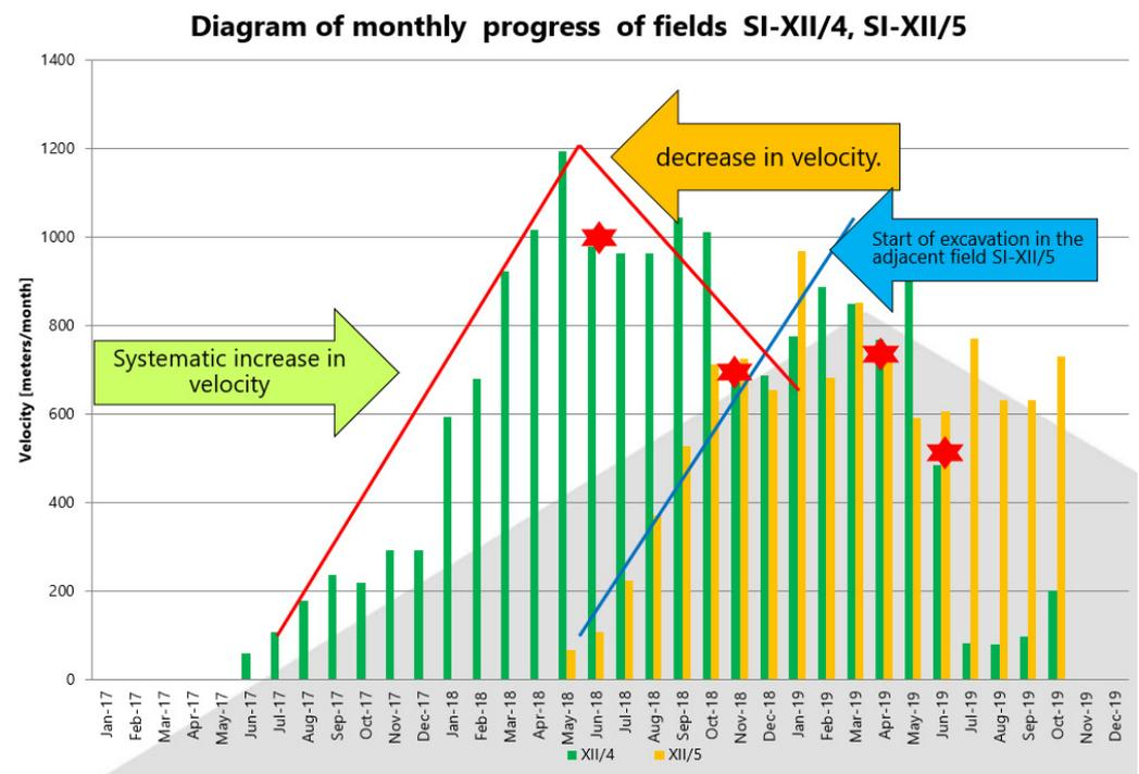
**Figure 4.** Diagram of the monthly velocity of the fields S-XII/4 and SI-XII/5. Red and blue lines are the limits of excavation velocity. Stars represent the moments of escalation of gas and the outburst hazard.
