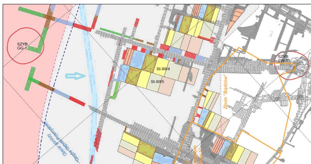
**Figure 1.** A map of the planned excavation in the areas of the projected hazard. Red circles—shaft location, orange line—salt deposit.
