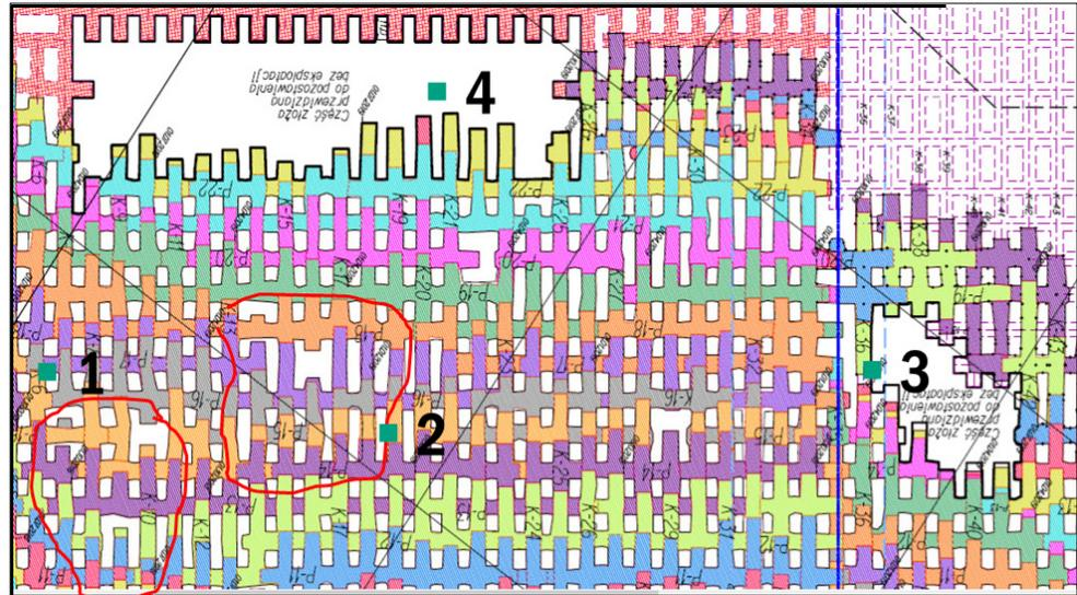
**Figure 2.** Sketch of the selected fragments of the fields, together with the progress of the individual excavation. White parts of the map signed in Polish mean parts of the mining field excluded from excavation. The colors represent the following months of excavation. The dotted lines symbolize the planned excavation of with room and pillar system.
