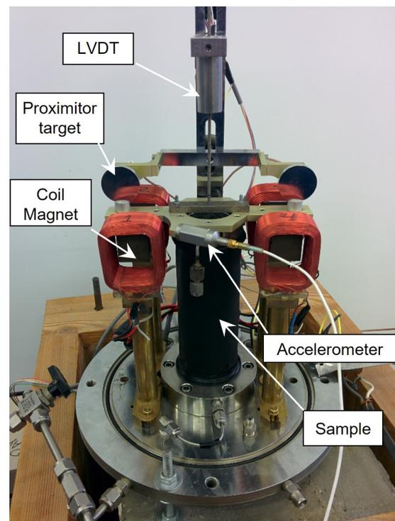
**Figure 2.** RC-TOSS testing device.
