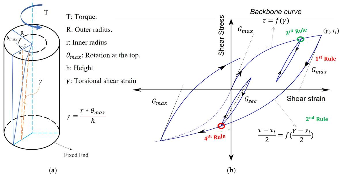
**Figure 1.** Concept for torsional strain in a fixed-free hollow cylinder specimen. (a) Diagram of the concept. (b) Hysteresis loop and Masing criteria.
