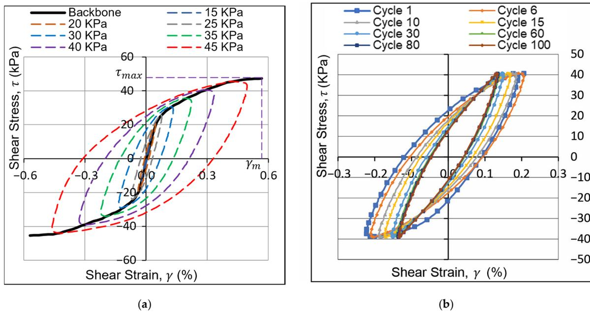
Figure 4. Demonstration of the types of conducted tests (results for Sample B, loose state). (a) Backbone curve test; (b) 100 TOSS cycles at 40 kPa shear stress.
