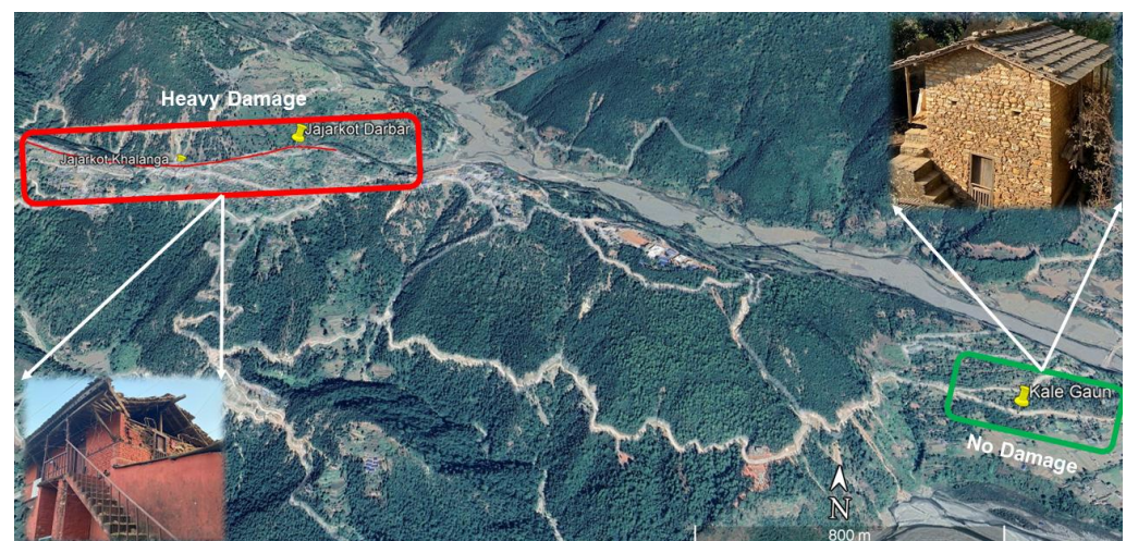
Figure 25. Damage in Khalanga, Jajarkot area indicating ridge effect due to earthquake.
