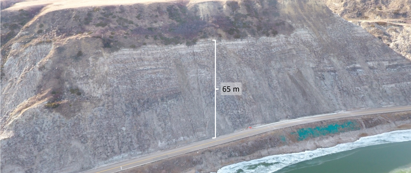
Figure S1: C018 – Red Deer River Valley Slope Instability – GSI and Joint Set
