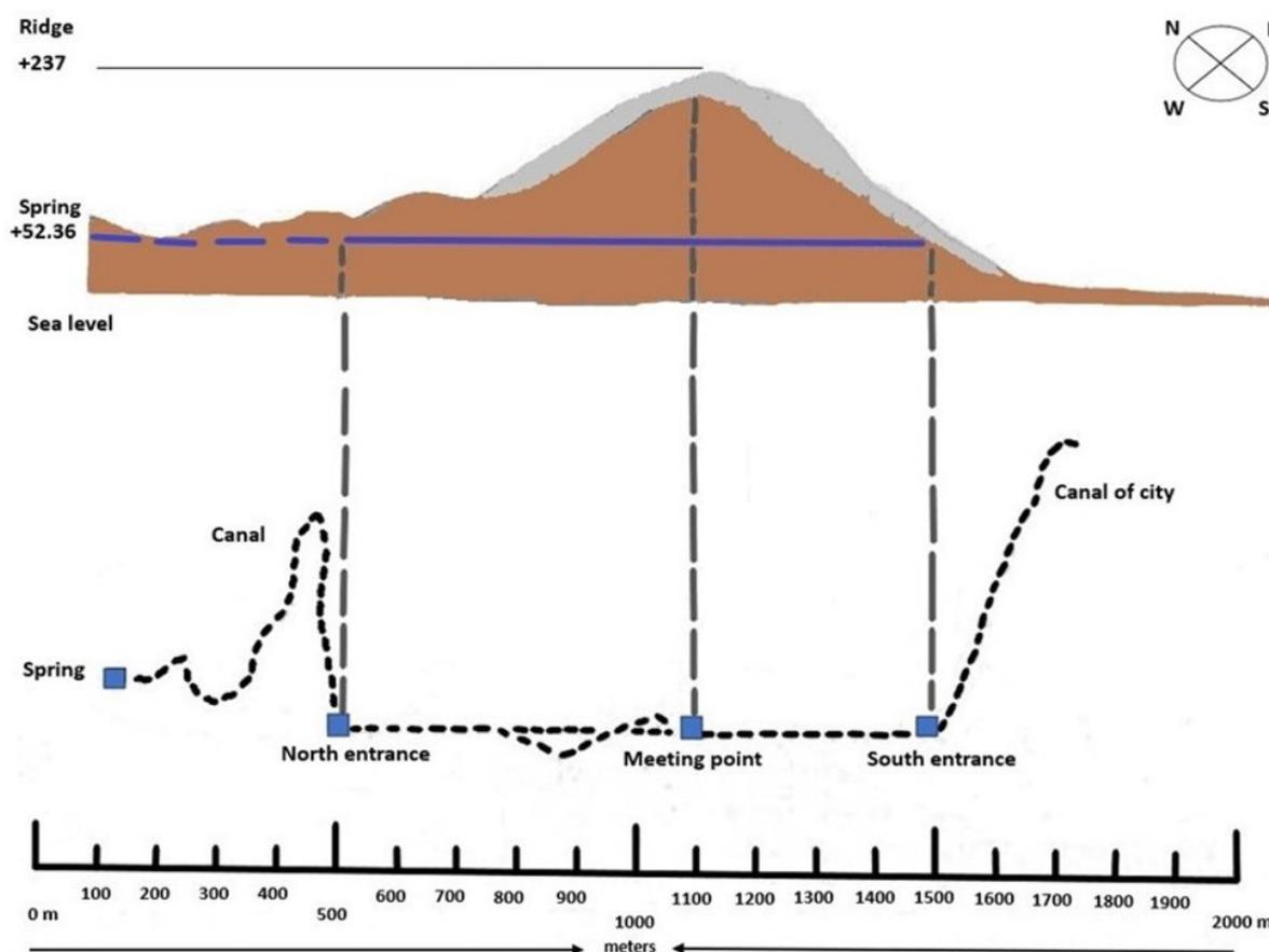
Figure 5. Simplified profile of the Eupalinos tunnel, [modified [38]].
