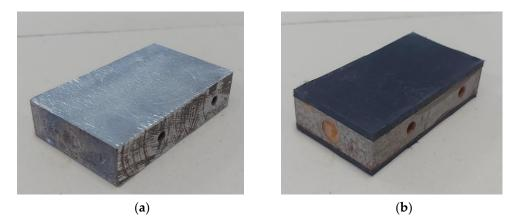
Figure 3. Uncovered steel pile model (a) and steel pile model with a *Reline* jacket (b).
