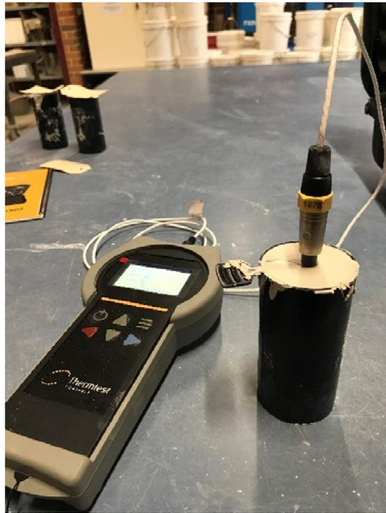
**Figure 3.** Thermal conductivity test.
