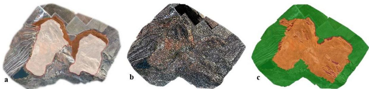
**Figure 7.** (a) Orthophoto overlaid by the reference data; (b) segmentation result; and (c) the final classification after refinement of the rule-based method for the RGB+DSM structure (green: non-affected, light brown: depletion, dark brown: scarp).
